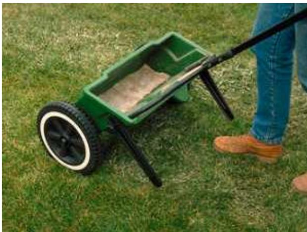
To ensure the proper amount of fertilizer is applied, *spreaders should be properly calibrated*. As spreaders get older, settings gradually change because of wear and tear. Regular cleaning and lubrication of the spreader will help it perform properly. Labels on fertilizer
